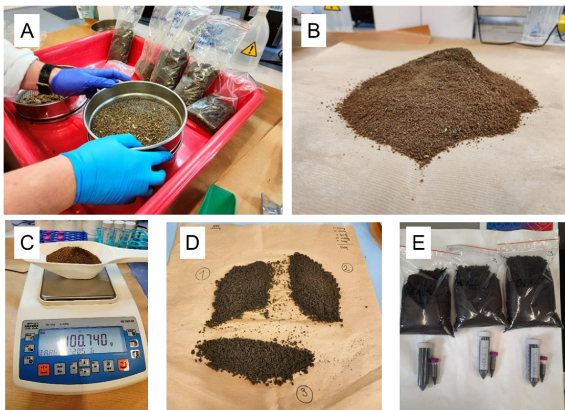
Figure 7. Soil samples preparation (A – sieving of soil sample, B – sieved soil sample, C – weighting of soil sample, D – soil samples divided into three technical replicates, E – soil samples in three type of containers)
